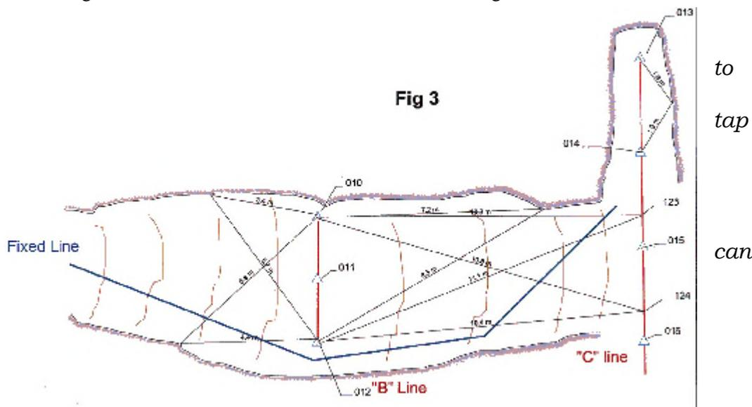
In the Pines survey this method suits ideally for the main chamber and the CCR. The link between the two sections will only in part incorporate some aspects of this method which is a point to point survey. Meaning the actual survey stations go in before the lines, based on a 3 dimensional line of sight. The skill requirement is more precise about where you put the survey points. It is not intended for Fred or Tom to do this.
